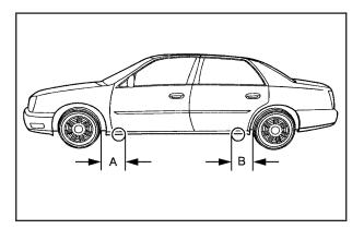
3. Find the jacking location from the diagram above and use the corresponding cutouts located in the plastic molding.
